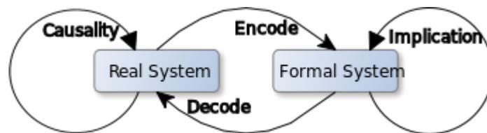
Modelling. On the left is a Real System with causal relations that we are trying to understand. On the right is a Formal System which is a representation of the real system on the left. Formal systems are constituted by their internal relations and so, when the behaviour of one component follows another, one will be able to draw formal implications within the system.
