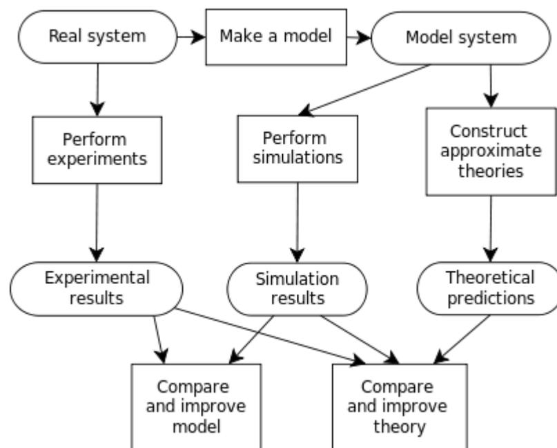
Simulations can therefore be thought of as virtual experiments, the outcome of which can be fed back into either the same model or theory in order to improve either or both. In the diagram at right the processes of experimentation, simulation and theoretical construction are depicted as running in parallel, though in practice, they need not.
